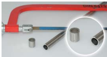
Result with a hacksaw (inside and outside burr)
